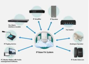
We offer all items of public announcement system along with seamless 3rd party integration to leading building & security management, CCTV, access control and telephony systems. Integration to SIP enabled digital telephone systems which allows users to make live announcements across the PA system from their telephone.
