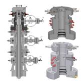
Tubing Head, the top spool on a surface wellhead, typically installed over the last string of pipe suspended in the well, the production casing
