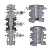
**Casing Spool,** a component that allows for an additional string of casing to be set in the well. Depending on the casing program for the well, there can be more casing spools
